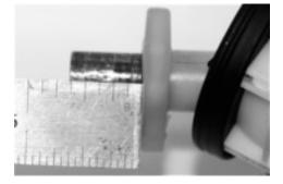
•Slip the new end on the base of the shifter. You May have to lightly tap it into place with a small hammer. Align the screws to third gear( front of the car as it is installed). Make sure to get it all the way up on the shifter rod. (shown left) Apply a small amount of thread locker to the setscrews. And snugly tighten them with the 3mm hex key.
