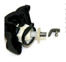
• First, we need to prepare the stock shifter to accept the new parts by cutting the end of the shifter off as shown in the image to the right. You need to make sure to cut it on the long side of 5/8" to leave the proper amount. De-burr the end of the shaft with a file so it will fit easily.
